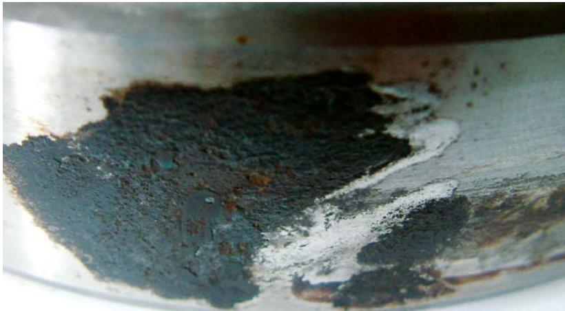
Fretting corrosion on the outer ring
